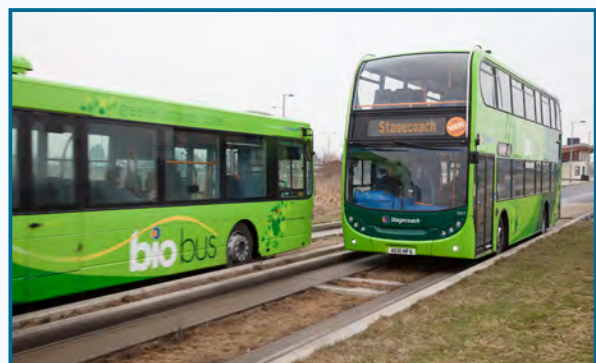
BRT – Bus Rapid Transit. Range of technologies involving full or partial segregation of high quality bus network away from other road users. Operation and performance more akin to light rail/tram rather local bus service with fewer stops/shorter journey times. In the UK The Cambridge guided bus way is perhaps the best example.
